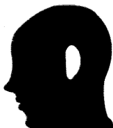
Fig. 2. A proposed 6 mm thick smooth lossy ear phantom to obtain peak 1- and 10-g SARs within \pm 10\text{-}15\% of those obtained for anatomically-realistic models. This model with the lossy ear replaced by a 6 mm thick plastic ear ( \epsilon_r = 2.56 ) gives SARs that are a factor of 2 or more lower as given in Tables 2, 3.
