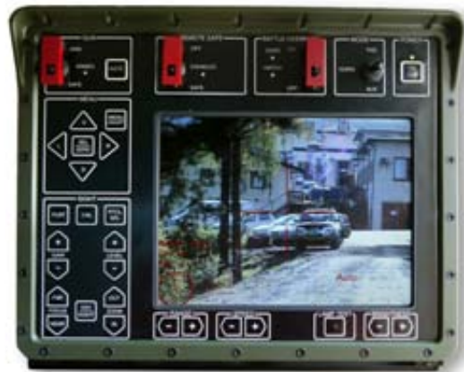
Fire Control Unit (FCU)
