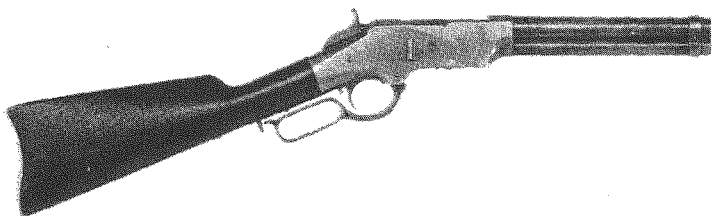
ORIGINAL PATENT MODEL with King's improvement, 1866. (Loading gate in side of receiver).
