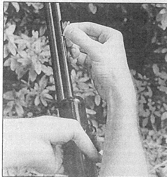
Many 22-caliber rifles with tubular magazines under the barrel have a loading port through which cartridges may be loaded.
