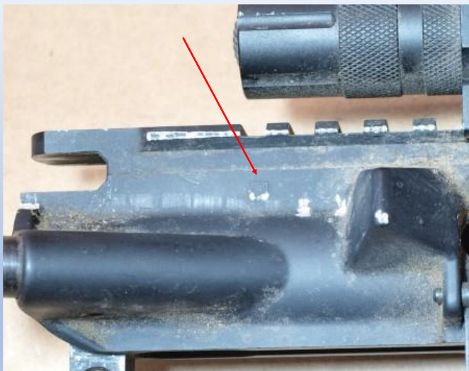
Evidence Upper #2 TCSO# 379-2 (E4) Forged Upper Receiver – “Incomplete”
