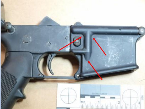
S1-36 Forged Lower-Evidence AR15 Rifle#1 (E2)
