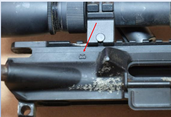
Evidence Rifle DOJ-9 (E5) Forged Upper Receiver
