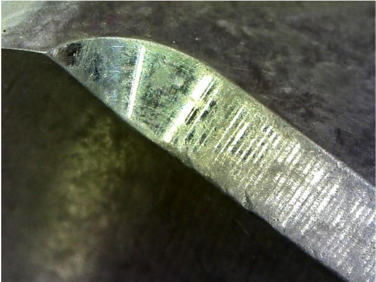
Front Corner of Forged Lower is Radiused
