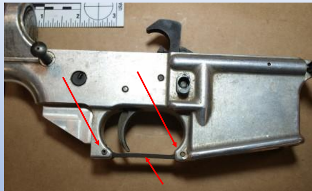
379-2 Forged Lower- Incomplete Evidence AR15 Rifle (E4)
