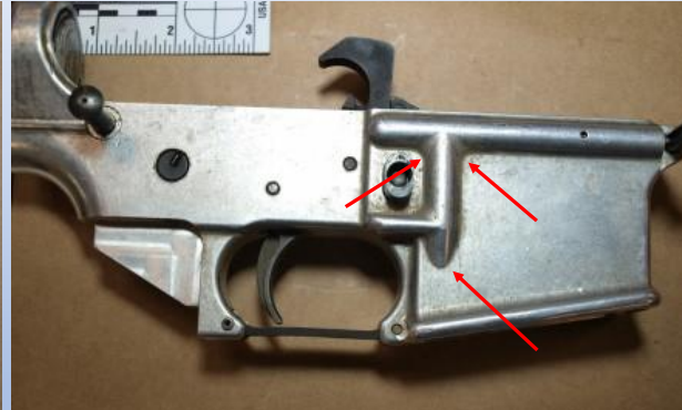
379-2 Forged Lower- Incomplete Evidence AR15 Rifle (E4)
