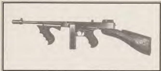
The top-slotted Cutts compensator was added to the muzzle of the M1928 Thompson submachine gun to reduce muzzle climb by expelling gas upward each time a round was fired. (Collection of the author)
