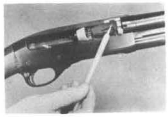
Cut away view showing breech block locked in barrel extension. A Remington exclusive feature on pump guns.
