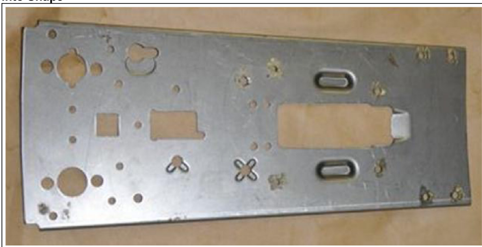
Figure 8: A Flat with All of the Required Holes Drilled but That Has Not Been Bent into Shape
