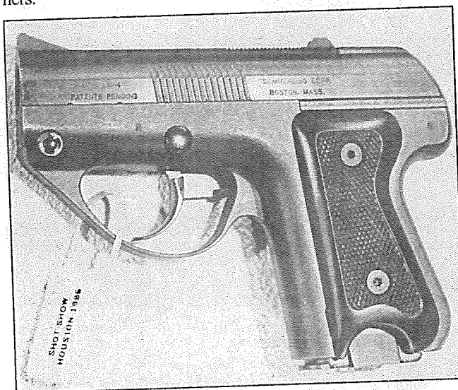
This Semmerling LM4 is one of the few manually operated repeating pistols produced in recent times. It is in 45 ACP and must be cycled by hand for each shot.
