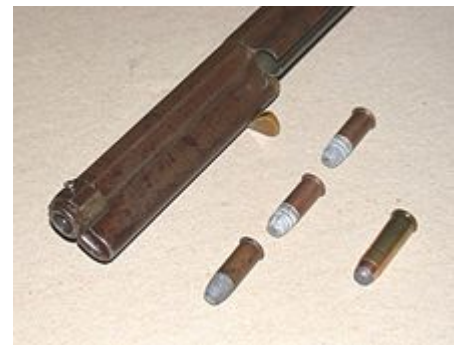
Loading sleeve open, three Henry Flat cartridges, compare with .44 WCF round
