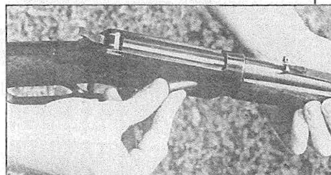
Most centerfire lever-action rifles load through a loading port in the right side of the receiver. This is a 30-30 Winchester Model 94.
