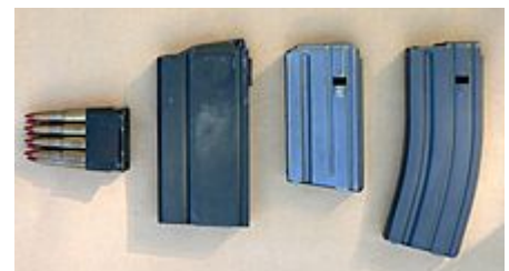
(left to right) M1 Garand 8-round en bloc clip, M14 20-round magazine, M16 STANAG 20- and 30-round magazines
