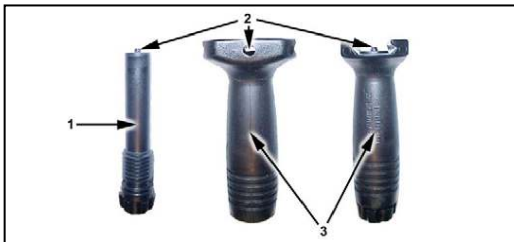
Figure 2-17. Vertical pistol grip.
