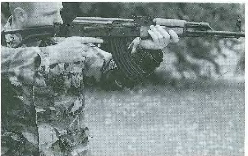
The sight radius of the AK is shorter than that of the AR and the rear sight is much farther from the eye than with the AR sights. Proper hold can be uncomfortable.
