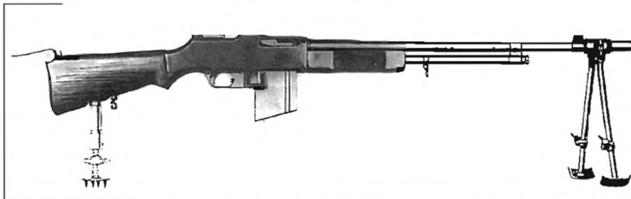
A complete M1818A1 Browning Automatic Rifle (BAR). This example is complete with the rear monopod, an item almost always removed by the user in the field.
