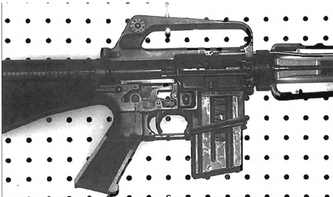
A rare cutaway AR-15 rifle from the Colt Gun Room. This photo shows all of the major internal workings of the AR-15/M16 weapon system. The hammer is forward in the uncocked (fired) position. PHOTO CREDIT: KEVIN DOCKERY/KNIGHT ARMAMENT COMPANY
