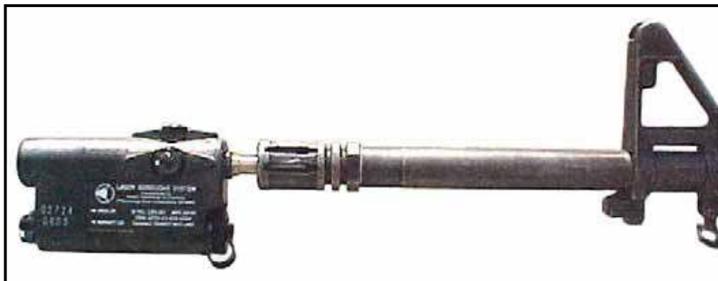
Figure 8-4. Borelight in the HALF TURN position.
