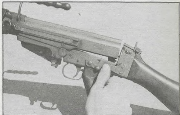
No tools are required to field strip the SAR-48. One presses locking lever straight up with the thumb, then pulls butt and trigger group down; it then swings open.
