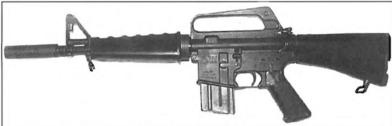
A left-side view of the Colt Model 07 CAR-15 submachine gun. The weapon is loaded with a 20 round magazine and the sliding buttstock is in its fully-forward position. The selector lever, directly above the pistol grip, is set to the semiautomatic fire position. This specimen has the longer, second type noise/flash suppressor.
