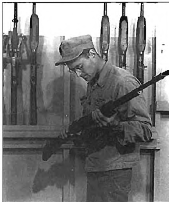
A technician checks an M1918 Browning Automatic Rifle (BAR) while on board ship in the Pacific during World War II. These early-model BAR's could still be found in Navy arms rooms throughout the war where they were used for ship defense and to arm landing parties. The last weapon on the left is an M1918 BAR with its forearm removed and a pintle adaptor installed. The pintle adaptor would allow the weapon to be placed in any standard machine gun mount on board ship.
