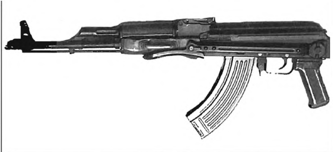
A left-side view of a Soviet AKMS-47 with its stock folded. The pattern seen just above the buttplate on the wooden foregrip is distinctive of the laminated wood used in many Soviet Block-produced AK-47 series weapons. PHOTO CREDIT: KEVIN DOCKERY
