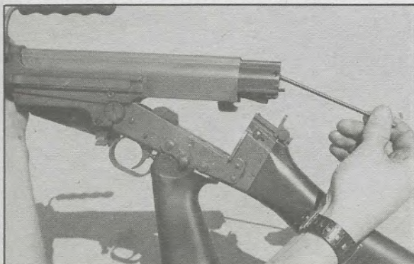
Remove the entire breech block and slide assembly by gently pulling the slide rod that is hinged to slide.
