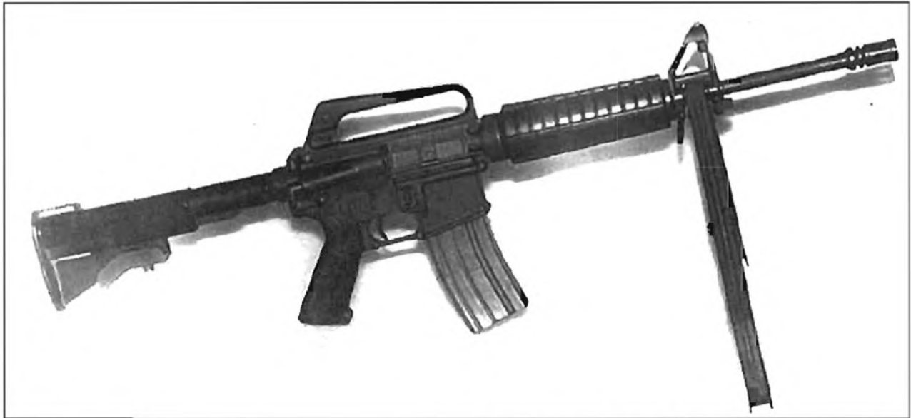
A right-side view of the Colt Model 653 carbine. The buttstock is in the maximum extended position and the weapon is loaded with a production 30 round magazine. The forward bolt assist can be seen on the upper receiver just above the pistol grip. The spring-loaded ejection port is closed in this picture. The weapon is supported by an M3 bipod clamped below the front sight and the muzzle is mounted with the third model "birdcage" flash suppressor.
