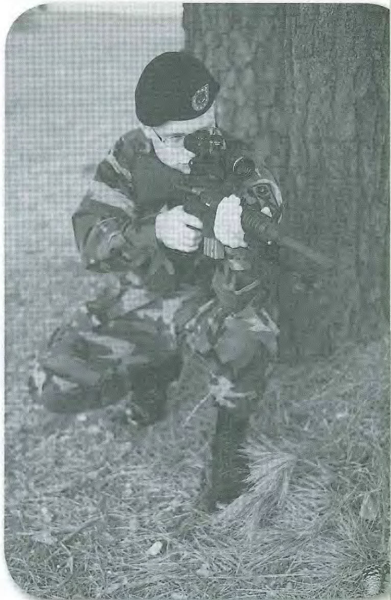
Here the Bushmaster has been outfitted with the ATN illuminated reticle scope. This scope can be set for 100, 200 and 300-yard targets by click adjustments.
