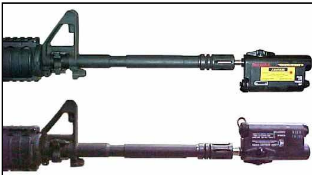
Figure 8-3. Borelight in the START POINT position.
