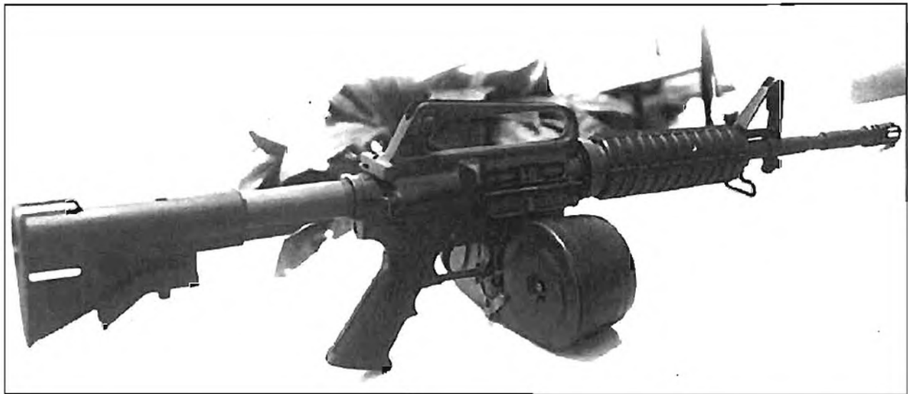
A Colt Model 723 Carbine with its sliding stock in the fully-extended position. The weapon is loaded with a C-MAG 100 round double-drum magazine. The C-MAG magazine holds 50 rounds on either side of the magazine well of the weapon and feeds rounds alternately from each drum as the weapon is fired. The low-silhouette of the C-MAG design is illustrated in this photograph. The notch around the barrel of the Model 723 carbine is for the mounting of an M203 40mm grenade launcher without further modification to the carbine or launcher. PHOTO CREDIT: KEVIN DOCKERY
