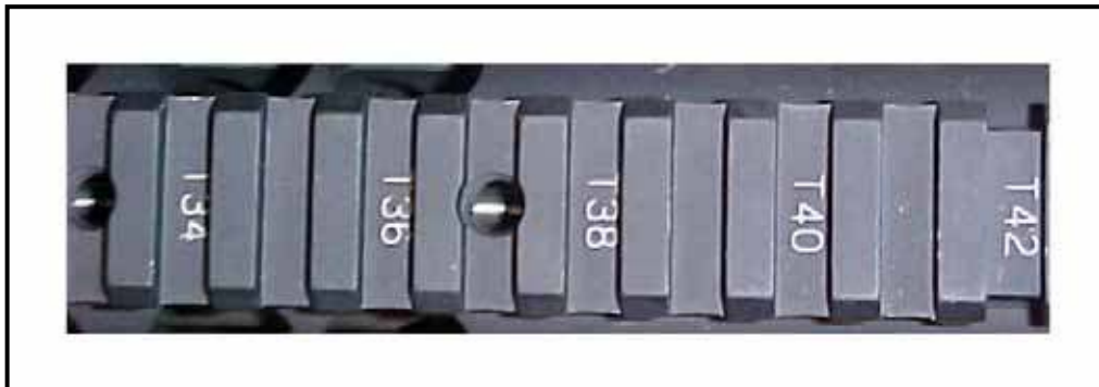
Figure 2-16. Address markings on RAS.
