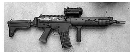
The final version of the Ak 5C with an Aimpoint red dot sight and forward vertical grip
