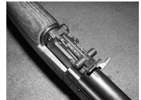
Rear sight of a Chinese Type 56, featuring 100 to 800 m (109 to 875 yd) settings and omission of a battle zero setting
