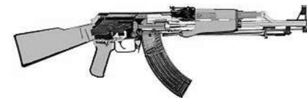
The gas-operated mechanism of a Norinco AK-47
