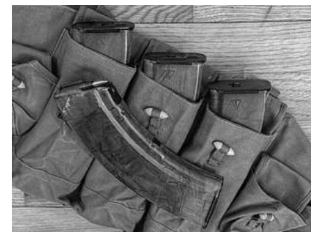
"Bakelite" rust-colored steel-reinforced 30-round plastic box 7.62×39mm AK magazines. Three magazines have an "arrow in triangle" Izhmash arsenal mark on the bottom right. The other magazine has a "star" Tula arsenal mark on the bottom right
