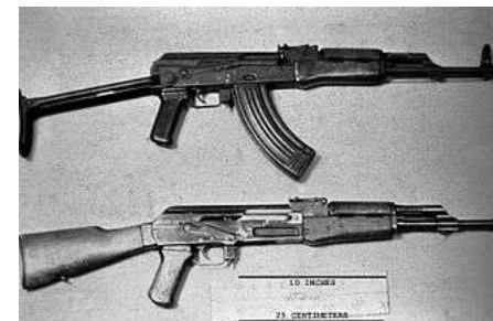
AKMS with a stamped Type 4B receiver (top) and an AK-47 with a milled Type 2A receiver
