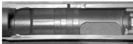
The barrel locks into locking recesses in the underside of the slide similar to that of an M1911-type pistol.
