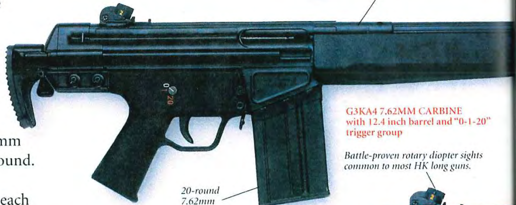
The G3K is a compact carbine-sized weapon firing the full power 7.62 x 51mm cartridge.
