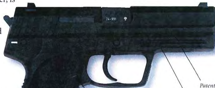
The ambidextrous magazine release lever is shielded by the trigger guard from inadvertent actuation. It can be easily operated using the thumb or index finger without adjusting the grip of the firing hand.
