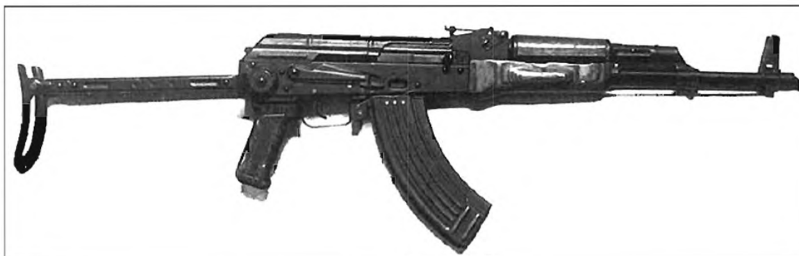
A Soviet-bloc produced AKMS-47 rifle with its folding stock extended. The long selector lever, above the trigger, is set to the mid-position for full-automatic fire. This specimen has the standard laminated wood forend and a plastic pistol grip. PHOTO CREDIT: KEVIN DOCKERY
