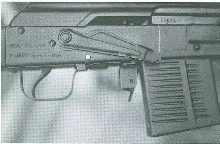
The Saiga rifle is a beefed-up AK firing a 308 cartridge. The safety is up and on, locking the bolt. In the down position, the rifle is ready to fire. Campbell contends this is certainly not the handiest of modern battle rifle safeties.
