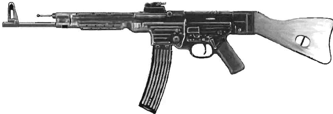
German rifles like this Sturmgewehr MP44, built cheaply by using modern industrial techniques, paved the way for later "assault rifles" that would be developed through the last half of the 20th century.
