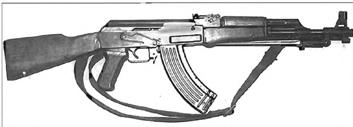
A right-side view of a late-model Chinese Type 56 rifle with a folding, spike bayonet. This is the Chicom version of the Soviet AK-47 and was the most common weapon of its type encountered by the SEALs in Vietnam. PHOTO CREDIT: KEVIN DOCKERY
