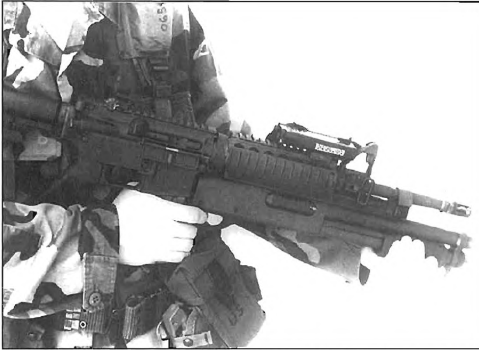
The M4A1 carbine with the Knight RIS system. Mounted on the top rail of the RIS forend is an infrared aiming light. On either side of the forend are "11 rib" full length handguard sections. On the bottom of the RIS, held in a firing position by the operator, is the KAC "Masterkey" shotgun, a modified 12 gage Remington 870 pump shotgun used primarily for opening doors by blasting off the hinges/lock.
