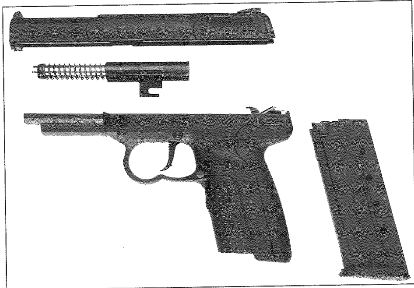
The Five-sevenN field-stripped; don't be fooled by the lug, this is a delayed blowback pistol.
