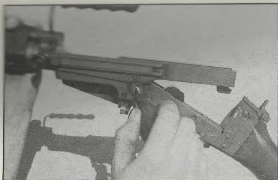
If one wants the separate barrel from the stock, small screwdriver or even cartridge rim can be used to turn the slotted screw head, thus allowing the disassembly.
