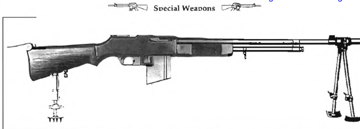
A complete M1818A1 Browning Automatic Rifle (BAR). This example is complete with the rear monopod, an item almost always removed by the user in the field.
