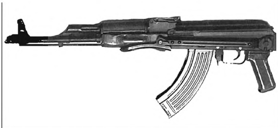
A left-side view of a Soviet AKMS-47 with its stock folded. The pattern seen just above the buttplate on the wooden foregrip is distinctive of the laminated wood used in many Soviet Block-produced AK-47 series weapons. PHOTO CREDIT: KEVIN DOCKERY
