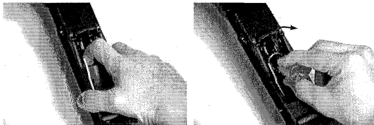
Figure F-1: Clear Double Feed by Rotating Shell Around Lifters
