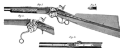
Diagram of the Spencer rifle showing the tubular magazine in the butt
