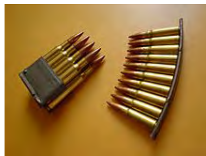
Comparison of M1 Garand en bloc clip (left), and SKS stripper clip (right)
