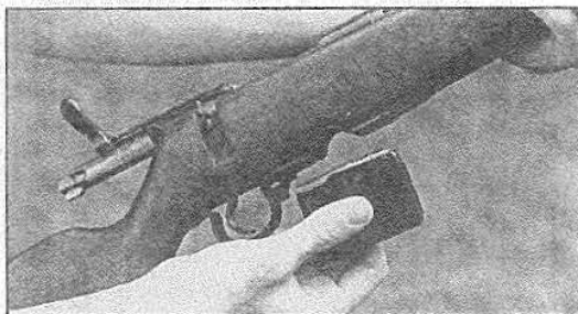
Some bolt-action rifles, such as this 30-30 Stevens Model 325, have a removable box magazine.
