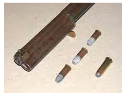
Loading sleeve open, three Henry Flat cartridges, compare with .44 WCF round
