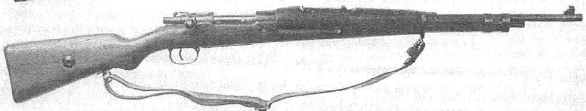
The Mauser '98 was probably the most important bolt-action rifle design ever produced. Many other designs are modifications of the Mauser '98. The basic design has a non-detachable magazine and can be loaded with single cartridges or from a stripper clip.
