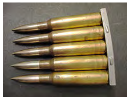
Swedish Mauser stripper clip loaded with Swedish 6.5×55mm
