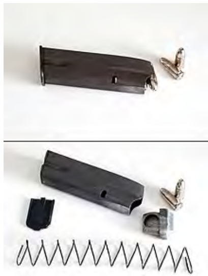
A staggered-column 9×19mm Browning Hi-Power pistol box magazine. The top image shows the magazine loaded and ready for use, while the lower image shows it unloaded and disassembled
