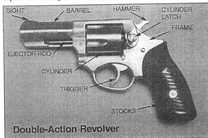
Fig. 112. A typical double-action revolver, showing some of the major features and components.
