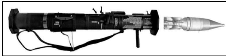
Figure D-2. M136A1 AT4-CS launcher and high explosive antitank cartridge
