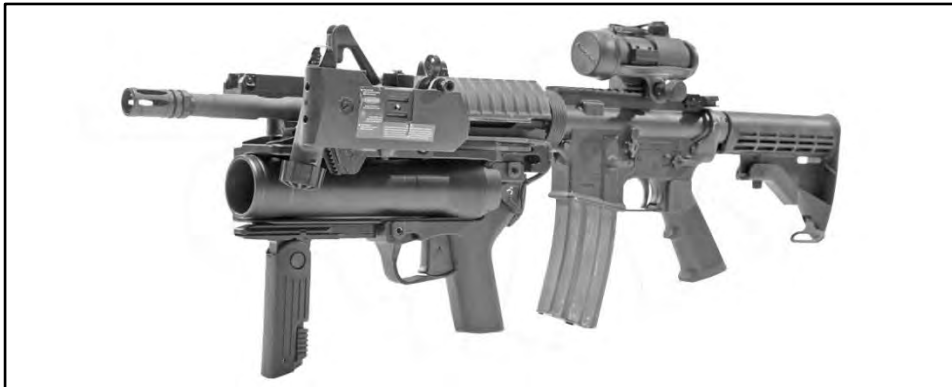
Figure 4-1. M320 attached to M4 series carbine example
