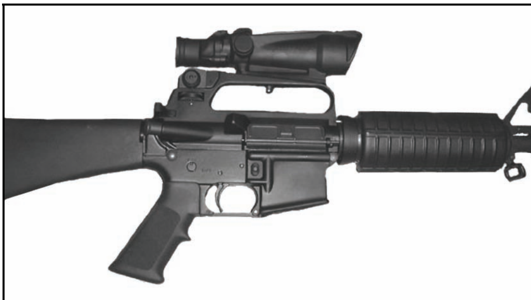
Figure 2-45. Mounting the ACOG on an M16A1/A2/A3 rifle.
