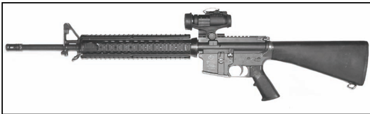
Figure 2-23. Mounting the M68 on an M16A4 rifle or M4-series carbine.
