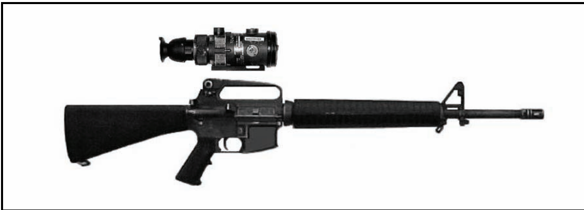
Figure 2-40. Mounting the AN/PVS-4 on an M16A1/A2/A3 rifle.
