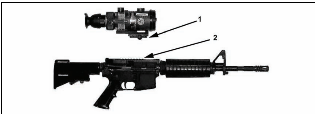
Figure 2-39. Mounting the AN/PVS-4 on an M4 carbine or M4 MWS.
