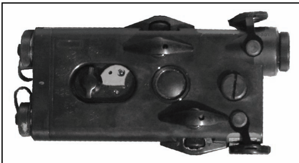
Figure 2-29. AN/PEQ-2A/B target pointer/illuminator/aiming light.
