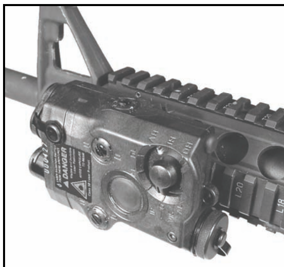
Figure 2-34. AN/PEQ-15 mounted on M4 carbine.
